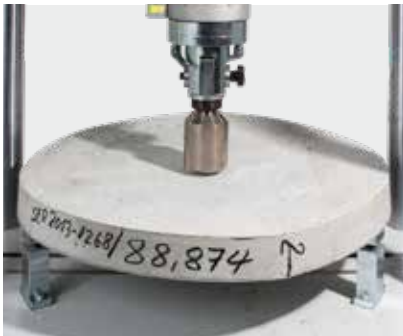
Round panel test: ASTM C1550
