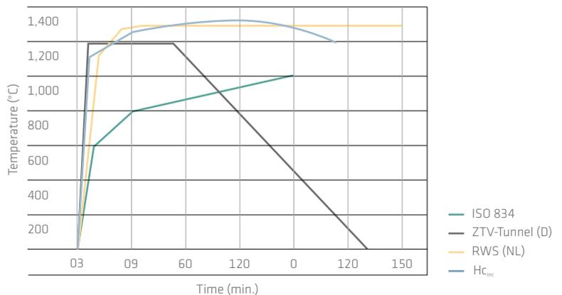
These fire exposure rating curves all simulate the temperature profile of a tunnel fire. The example of the Dutch RWS curve defines the maximum exposure which can be expected in the worst case scenario: This is defined as a fire of a road tanker truck with a load capacity of 50 m<sup>3</sup> that is 90% full of liquid hydrocarbon fuel (petrol).
