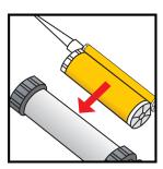
4. Place the cartridge into the gun and start application
