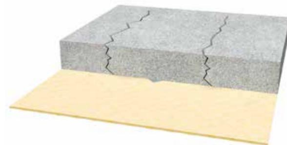
If non-bonded systems are damaged, water spreads uncontrolled between the membrane and the concrete. Water can easily enter every weak point of the structure, such as joints and cracks.
